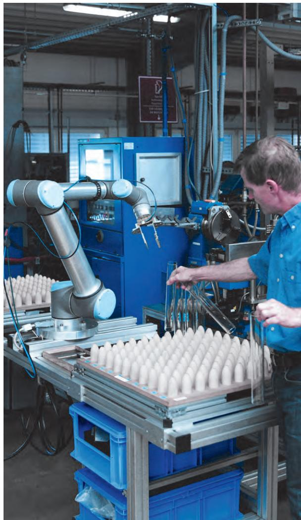
One smaller setup that has benefitted from deploying cobots is Multi-Wing CZ in the Czech Republic. The company manufactures axial fan solutions for ventilation applications and needed to automate production within a very confined workspace to meet growing demand. Removing its old safety guard and installing a UR5 cobot from Universal Robots enabled the company to cut per-unit production costs by 10–20% and boost capacity by 336 hours per year.
